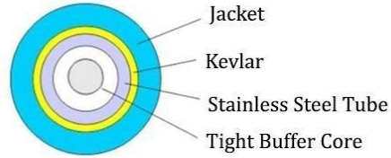
600um Color Coded Fiber, Kevlar, Inner Jacket, Steel Tube
